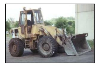
This older CAT 920 front end loader gets limited use each year. LE's 8800 Monolec Ultra Engine Oil is only changed with planned maintenance at 300 hours.
